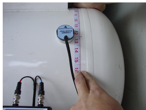
HANDHELD SENSOR EASILY DETECTS LIQUID LEVEL
