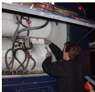
Fig. 5. Measuring the Maximus™ Detected Liquid Level after Refueling
